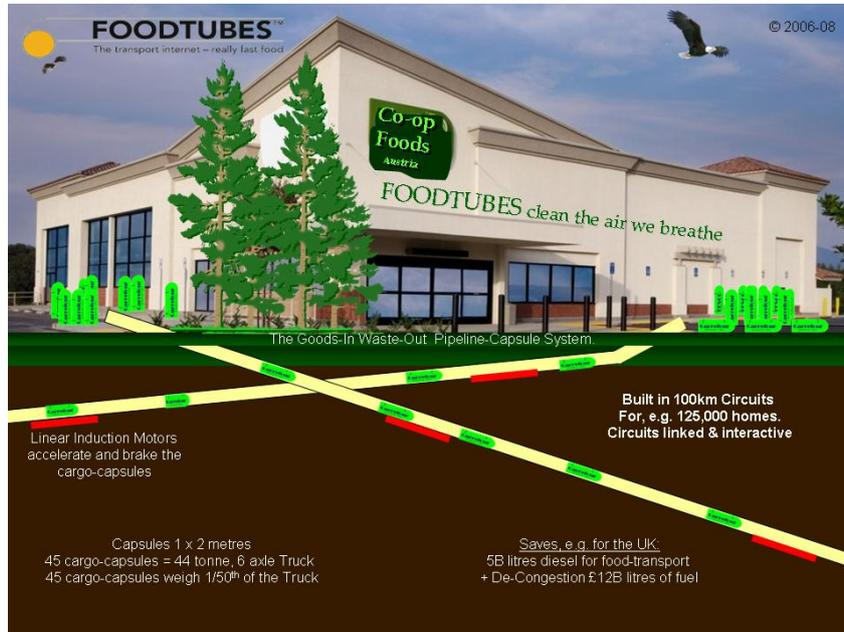
The Capsules will be precisely controlled by software – to travel through numerous interlinked, open-architecture Foodtubes Circuits, each of about 100 km; eventually forming **The Transport Internet™**.
