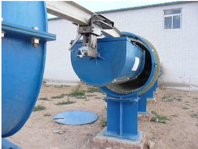
Figure 6 Capsules for the Magplane Technology Inc coal pipeline suspended from a test track[15]
