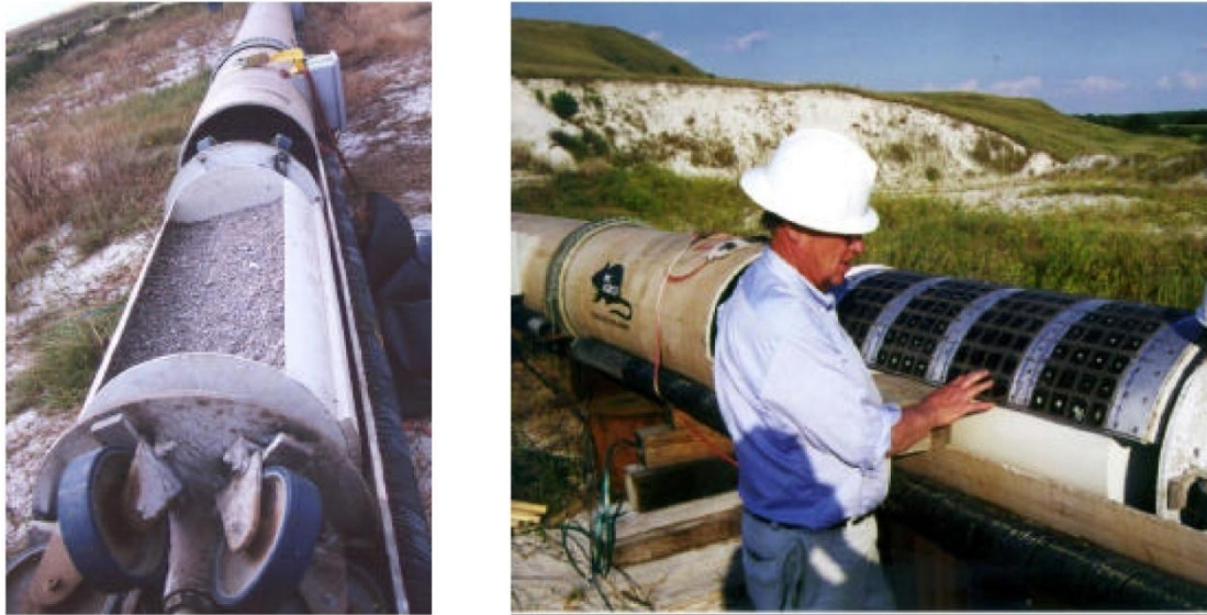
Figure 4: Magplane Technology demonstrator capsule carrying 300Kg of phosphate and the linear synchronous motor[10]
