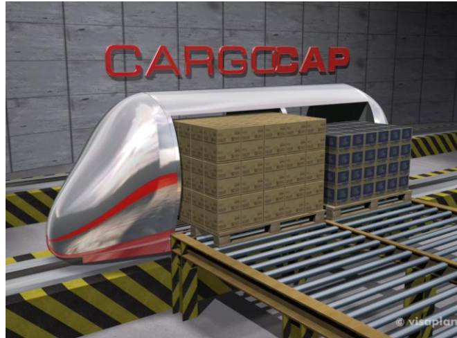
Figure 5: Artist impression of a CargoCap capsule being loaded with two Euro-pallets[13]
