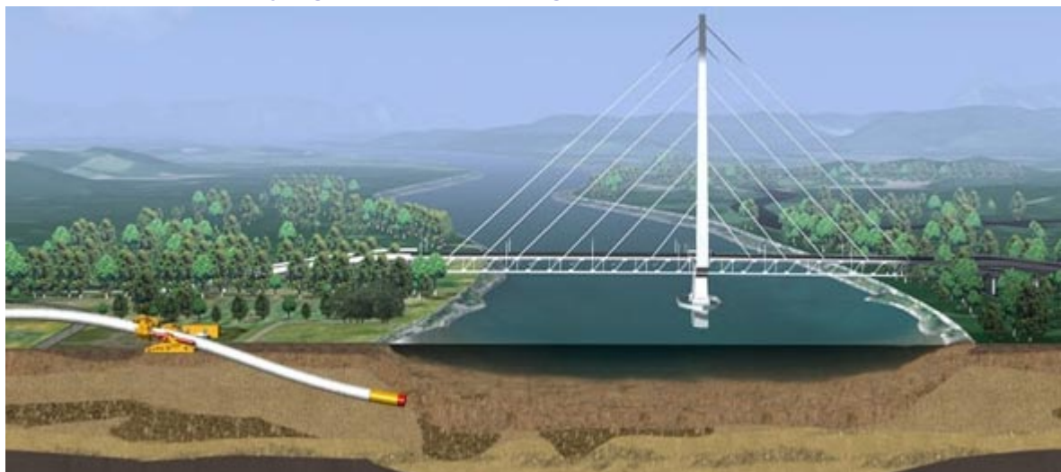
Figure 7 – Herrenknecht - No-Dig pipe-laying under a river
