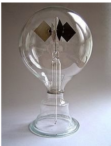
Crookes Radiometer. Paddles driven by light. In a vacuum
